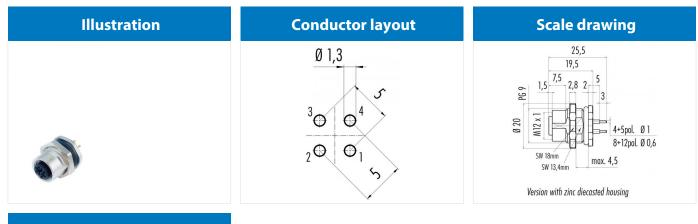
Contact arrangement (Plug-in side)
